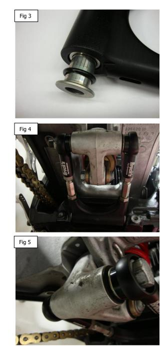
WARNING: Clearance between the OEM swingarm, pivot lever, and rear shock absorber is required for proper suspension travel. Following adjustment, check for clearance.
